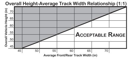
The measurements are to be taken from the ground to the tallest point of the vehicle for the Overall Vehicle Height and the normal track measurement as stated in Section 12 for the Average Track Width. (See figure on next page.)
