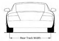
center of gravity above the road (H) and can be calculated by the formula SSF=T/2H. Vehicles with an SSF of less than 1.30 should not be permitted to compete in Solo® events due to the higher risk of rollover.
